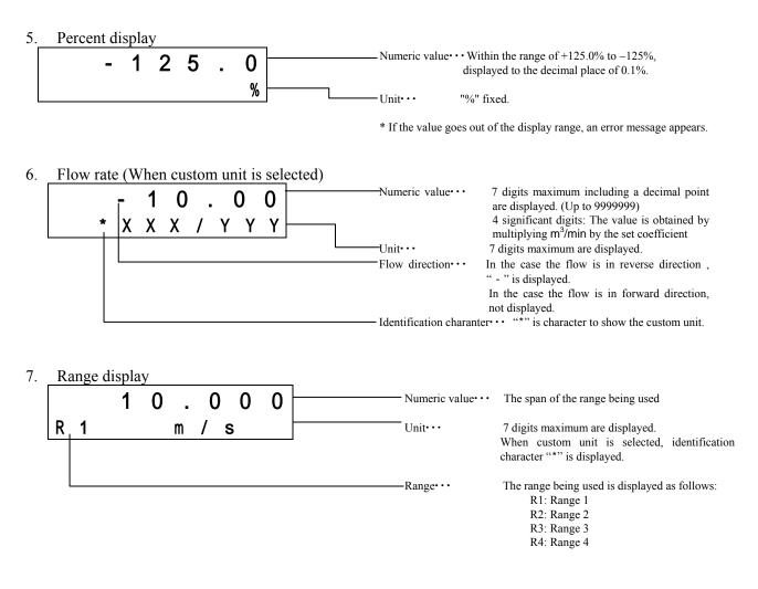
In the range display, the range currently used is displayed (any one of the ranges 1 to 4). The screen example above shows that Range 1 is currently used.
